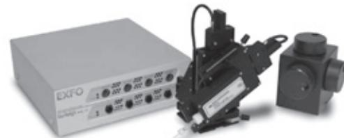
Extremely precise micromanipulator with motorized 5  $\mu$ m coarse and nanometer level, piezoelectric fine positioning
