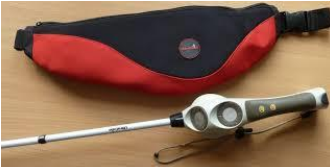
Ultracane: Distance to Vibration Intensity (Vibrotactile)
